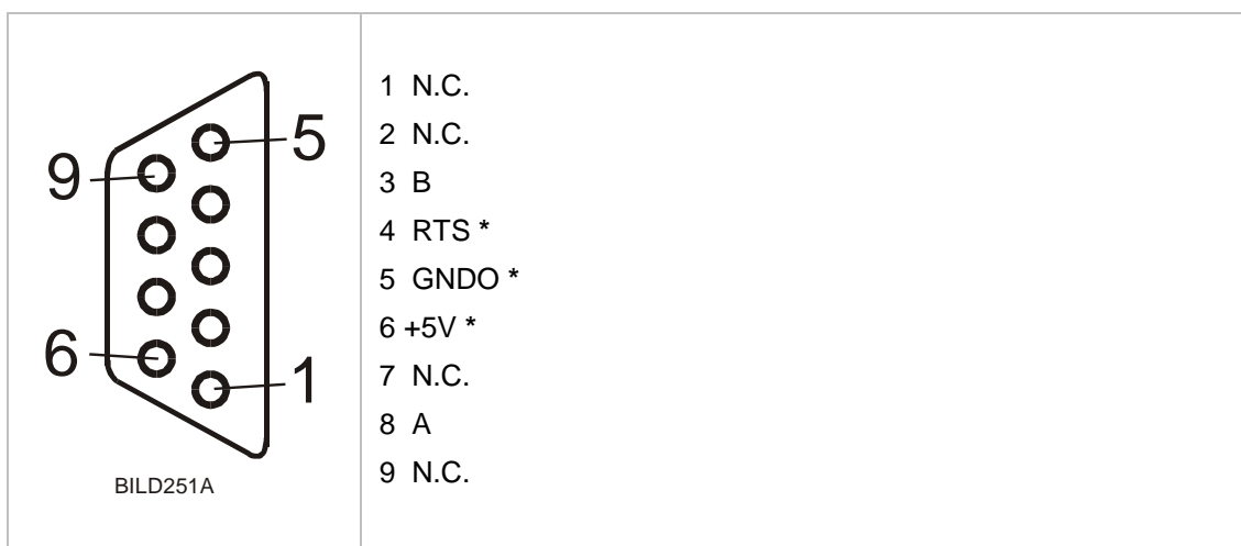
Figure 78: Connector Assignment (Sub-D, 9 poles, socket)
