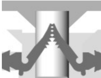
Figure 15: Sealing Lip System
